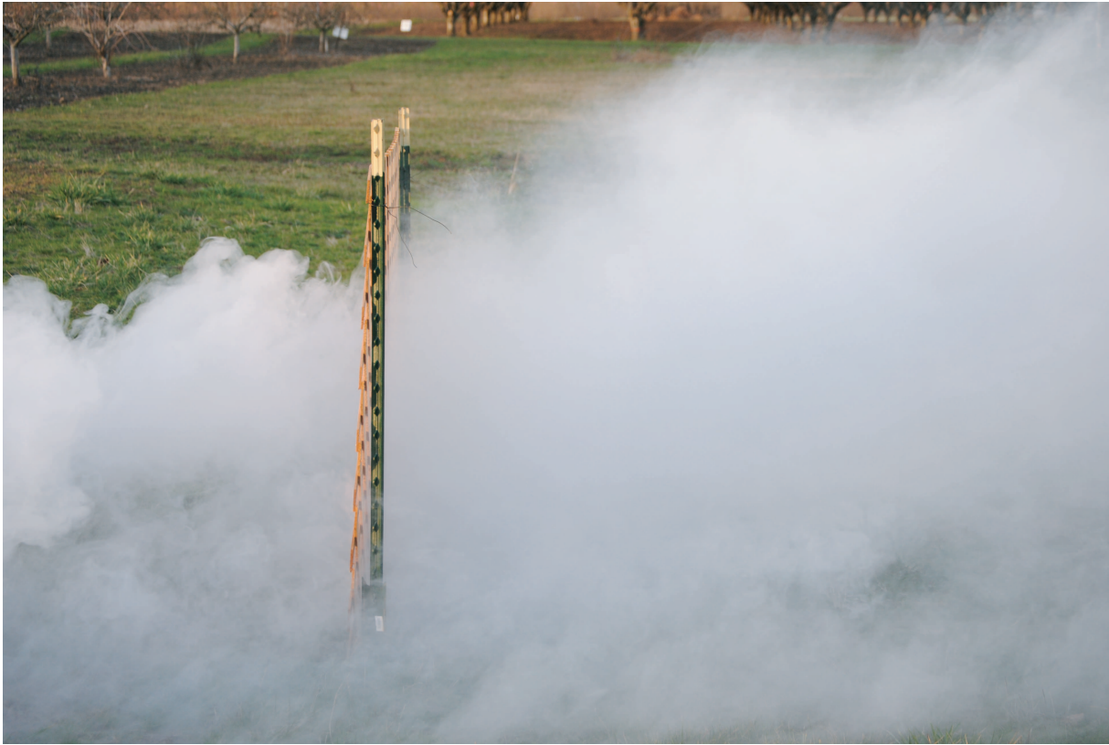
Figure 3: Flow from left to right. Notice that upwind turbulence near the surface seems fully developed but not near the top of the fog plume.
